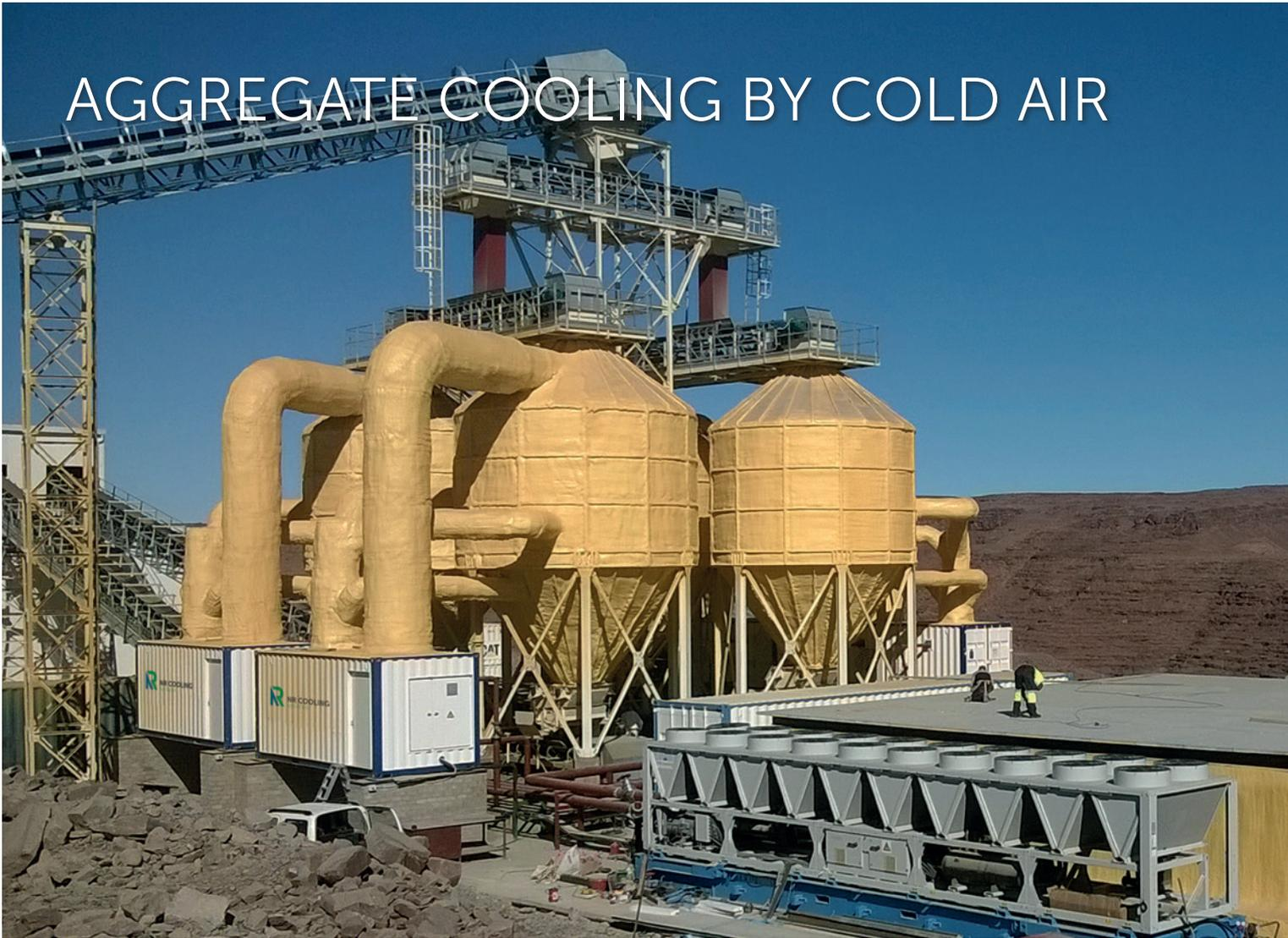
Concrete consists of 40% to 60% aggregate with sizes of 5 mm up to 150 mm. When high concrete production rates and extreme temperature reduction are required, cooling aggregate by air has proven to be very effective. When using this technology, the limitation of added water is not a limiting factor in reaching the desired concrete temperature. This means that lower concrete temperatures can be reached compared to other common systems.
