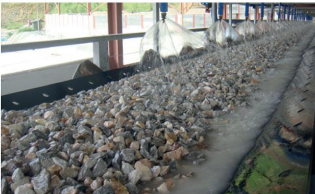
The cold water flows through the aggregate in opposite direction and is finally collected by a drip pan located underneath the belt. From this point the used water is transported to a sedimentation system for cleaning. After that the water is pumped back to the cooling plant.
